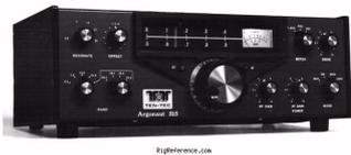
**Argonaut 515** (eHam.net rating 4.8/5) – released in 1978 the 515 is known as THE classic QRP transceiver, with enhanced band-spreading, 10m divided into 3 ranges, and slicker T-R switching. It instantly won popularity with DX operators and 36 years later is still used by many hams as their main station rig.
