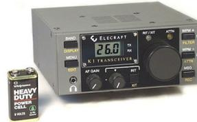
**K1** - A compact dual or quad-band CW transceiver with many of the K2 bells and whistles. It could be ordered with a choice of any TWO band modules, 80-15m, or if a FOUR band version was desired, provision could be made for 80, 40, 30, 20, 17 or 15m.
