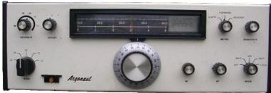
**Argonaut 509** (eHam.net rating of 4.8/5) - this model followed the 505 in 1973 and had improved circuitry plus the option of an external active CW filter. Again, Doc had several of these radios for DXing, contesting and local contacts. Originally the power supply was a pair of lantern batteries in series. Of course, there are a number of much more modern, efficient power sources available today!
