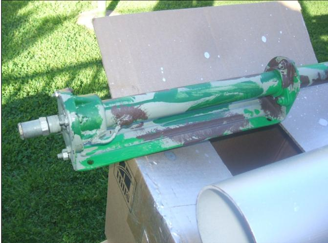
1. Modified Hy-Gain 18AVT base mounting section.
