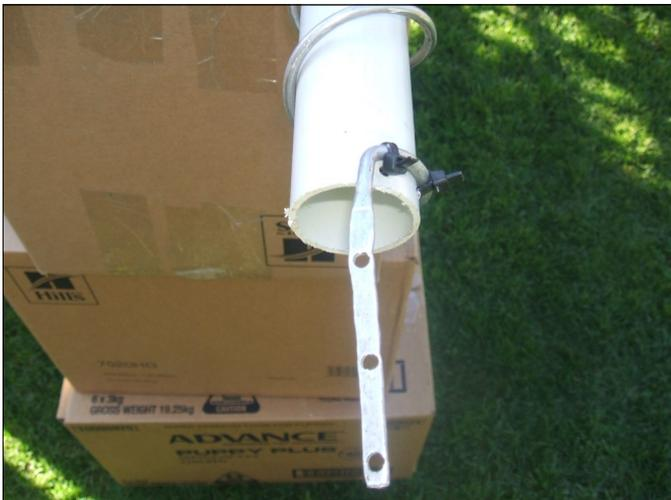
2. The top of the helix showing the flattened section of aluminium wire used for capacity hat connection.
