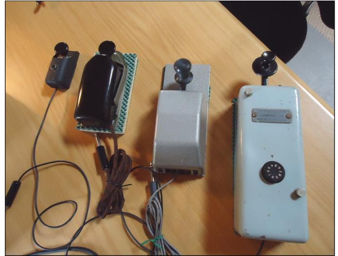
The picture above shows the difference in size of the four keys. From left to right: Jardillier, Czech, Junker and Marconi.
