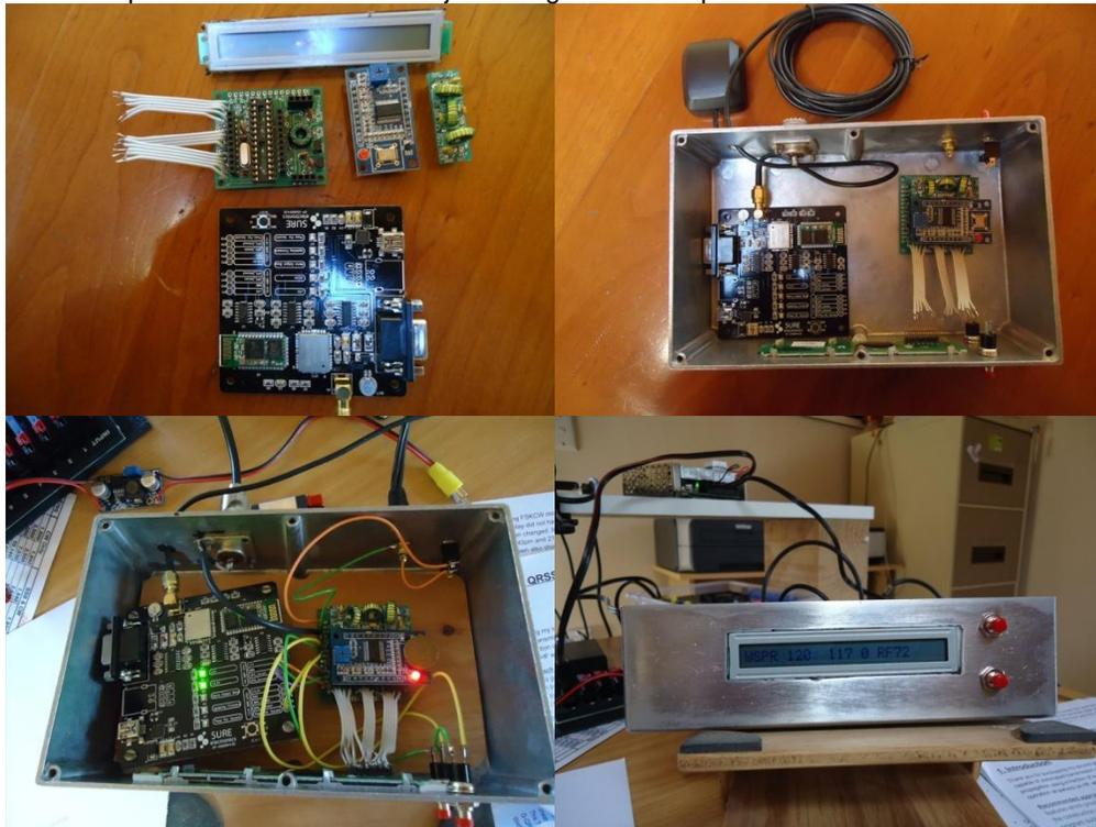
The WSPR software needs to have a very accurate clock for it to correlate with other wspr stations and the settings on the Ultimate 2 generally will stay in clock sync for few days. Therefore I bought on eBay (very cheap) a GPS board with an external antenna for keeping the kit adjusted to the exact time. That board is the black one marked Sure with the two green LED's. The kit needs to have a 5 volt power supply. Hans Summers can supply the full kit including the GPS etc.
