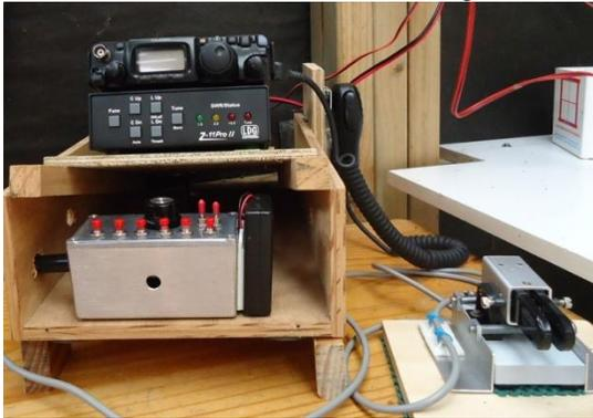
←The FT817 sitting on top of the LDG Proll tuner and underneath that is my CMOS III keyer with Galbraith paddle on RHS.
