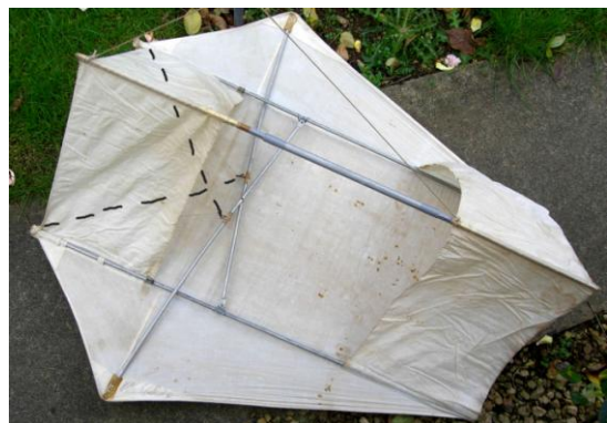
This photograph of the inside of a Wheelwrights Kite shows the similarity of the shape principle and the way in which the elastic bungee cords are fitted - but which are not actually fitted in this picture - They are indicated with the dotted lines showing how they tension the cross struts to keep the kite open when in flight..
