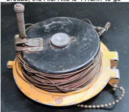
Business side of the original yellow dinghy rescue radio kite wire assembly that was built into the transmitter ( pictured in a fairly recent Keynote article) This holds around 200 feet of 1 mm diameter multi stranded woven copper wire
