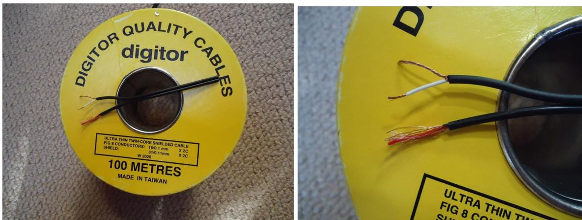
It is lightweight cable and very soft and subtle. The braid is not woven as in RG58 cable and is parallel with the insulated wire. It is perfect for wiring of keys paddles and speakers.
