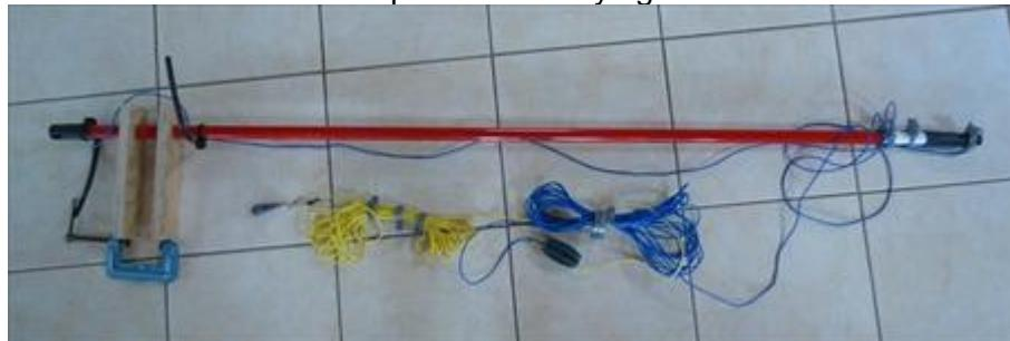
Some time ago I read an article on using an unun as opposed to a balun for a long wire. I built it using the plans of KC8AON's QRP projects. I mounted it in a plastic box and used loudspeaker spring loaded connections for attaching the antenna and counterpoises.
