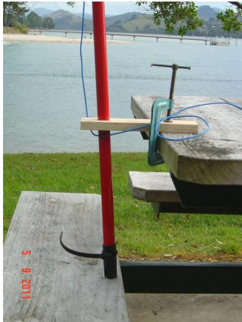
Method of clamping pole to table
