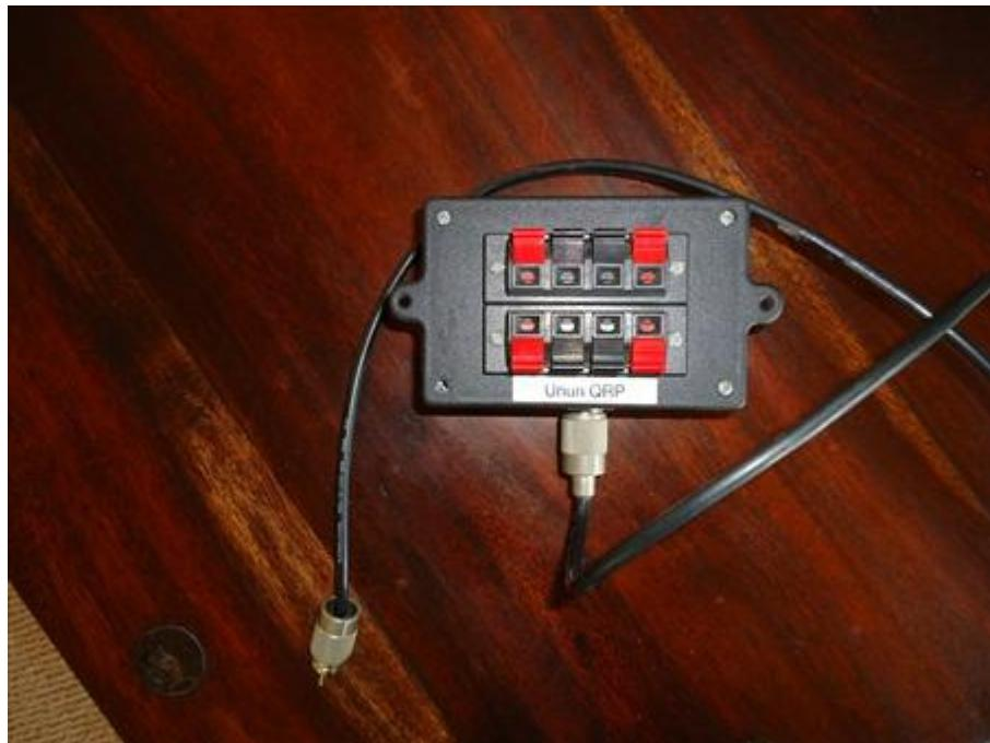
The counterpoises are just insulated wire cut to approximately a quarter wavelength on all the bands. The longest being 20 metres long for the 80 m band and the shortest being 2.5 metres long for the 10m band. I bound them together so that they don't get tangled up and soldered them all together at one point for inserting into the unun box. The counterpoises I lie along the ground in a straight line in such a way that they won't trip up any visitors.
