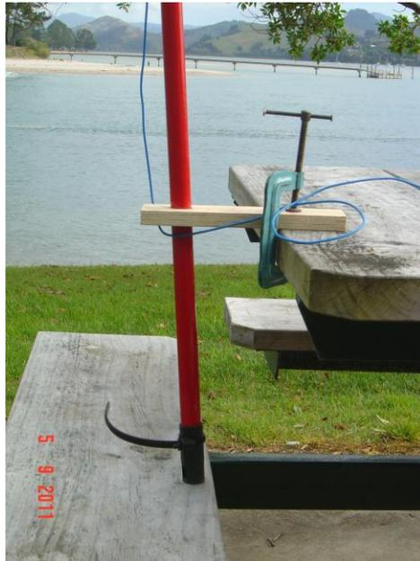
Method of clamping pole to table
