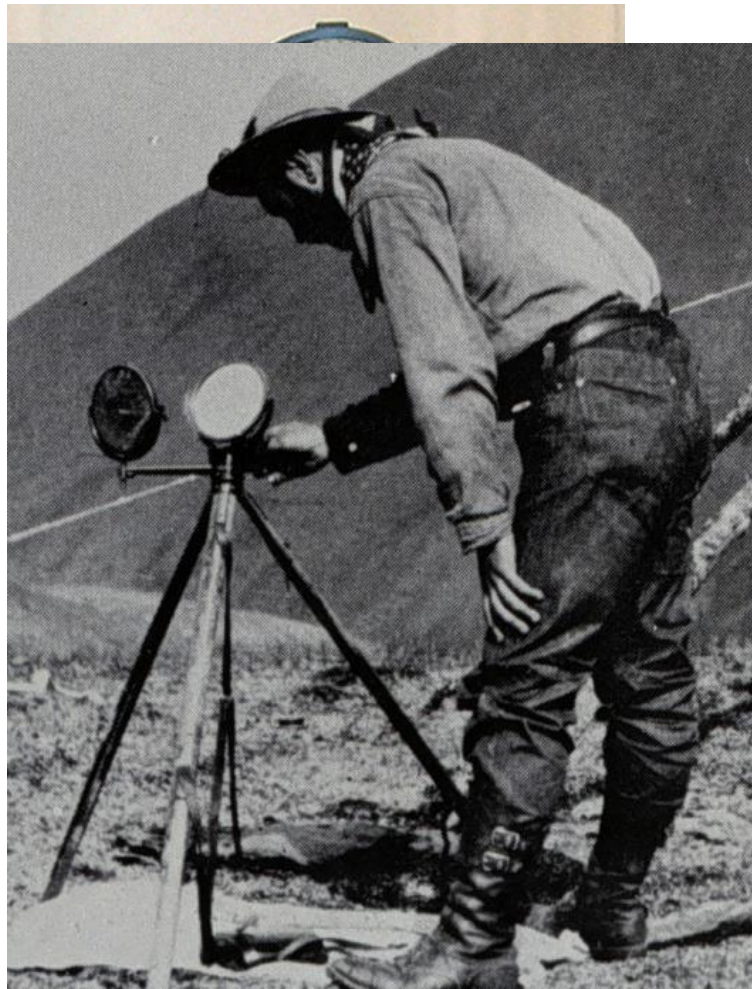
Fig. 2: German heliograph made by R. Fuess in Berlin (on display at the Museum of Communication in Frankfurt)
