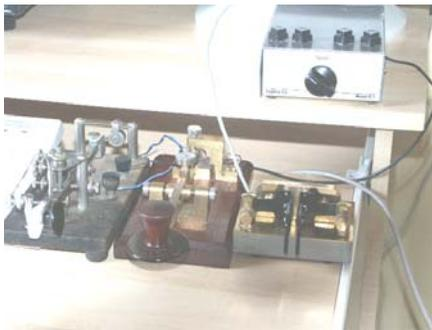
Hi Robert, as promised, a photo of me with the station used in SKW, the key is a copy of the GPO coast station keys. The other keys in use are a rather battered J36 bug and a twin paddle made by David VK3DBD/G3SCD, which I use via a Logikey K-1.
