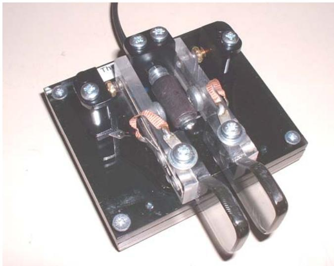
To complete the base and to make it heavy and to give good stability I used 3rd and 4th layers of sheet lead and final layer is sheet aluminium for strength. Sprayed black and with rubber feet it seems to work very well.
