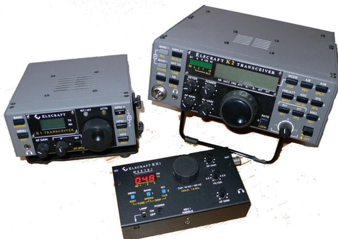
The third kit I built was the new KX-1, it's a dual band transceiver in its standard form on 40/20m , mine has the new 80/30m option too giving it 4 bands, its not much bigger than a packet of cigarettes but has a built in Auto ATU, Keyer, and battery pack. It really is a amazing bit of kit, the price to pay for such a small package is relatively low power, just over 1 watt
