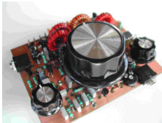
The Brent is a Direct conversion radio that gives around 1.5
