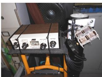
Left: Series broadcast capacitor to extend the Z matching of the MFJ coupler.
