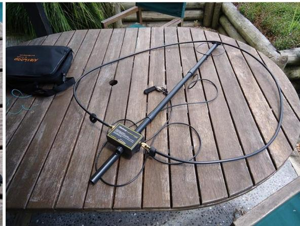
With the other loops that I have played with the exciter loop has been on the bottom and the capacitor was on the top. Alex has it the other way around and for good reason. The tuning capacitor is then at the correct height for it to be easily tuned by hand whilst sitting beside your radio.
