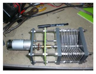
I have since motorised the capacitor, and now just need to box it up, weatherproof it, then relocate outside.
