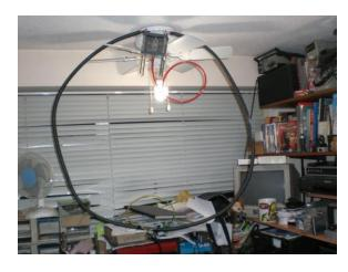
On the Antenna front, I have constructed a Magnetic loop over the last few weeks. I made the butterfly Capacitor, and got it working for the 11th Nov Ladder.
